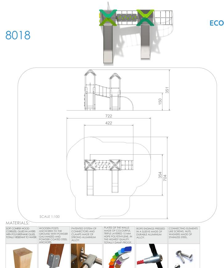
SUDES MADE OF STAINLESS STEEL AISI 304, METAL SHEET WITH A THICKNESS OF 2 MM FORMED IN A CNC TECHNIQUE. ANTI-SLIP ANTHRACITE 10MM HPL PLATFORM PLATE WITH A VERY HIGH RESISTANCE TO WEATHER CONDITIONS AND ATTRITION.
